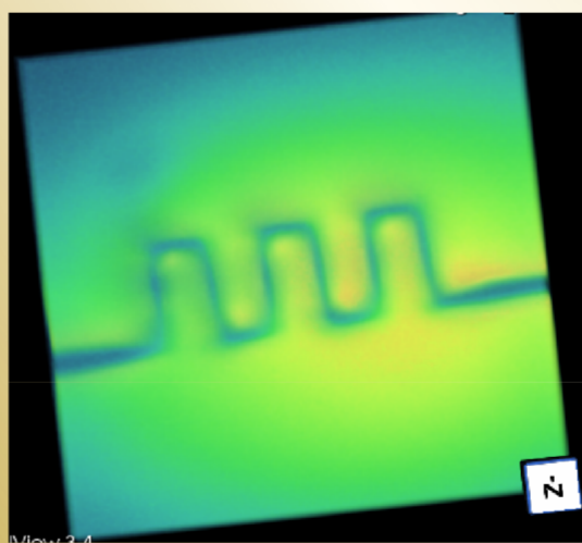
3D image of a PMG microchannels recorded by NLM
